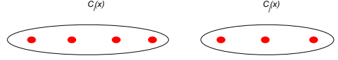
Fig. 1. Two maximal-confidence clusters C_i(x) and C_j(x) . The distance between two adjacent nodes in C_i(x) (or C_j(x) ) is not bigger than the maximal confidence bound of C_i(x) (or C_j(x) ), while the distance between these two clusters is bigger than the maximal confidence bound of C_i(x) and C_j(x) .
